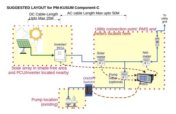
ii. RMS should have provision to give remote On/Off command to pump through farmer mobile app. to save ground water.
